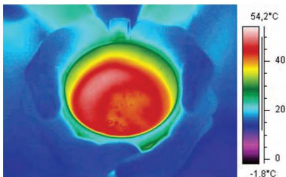
A thermogram shows the various temperatures of hands holding a hot drink. The heat radiation is detected electronically and displayed with different colors representing different temperatures.
