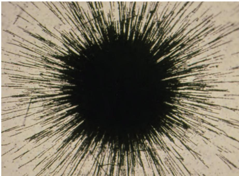
**Figure 7.4** Radium salts are placed on a photographic plate. After the plate is developed, the photograph shows the dark traces left by radiation emitted by the radium salts.
