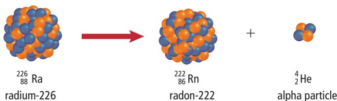
**Figure 7.10** The nucleus of an atom of radium-226 contains 88 protons and 138 neutrons. A radium-226 nucleus undergoes alpha decay to form a different element, radon-222, and an alpha particle.
