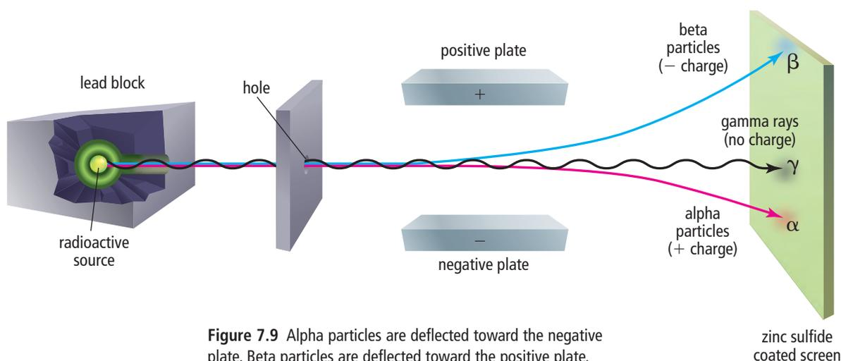
Figure 7.9 Alpha particles are deflected toward the negative plate. Beta particles are deflected toward the positive plate. Gamma radiation is not deflected by the electric field.
