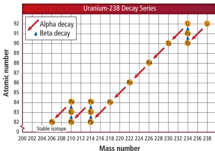
Figure 7.7 Uranium-238 undergoes 14 different radioactive decay steps before forming stable lead-206.
