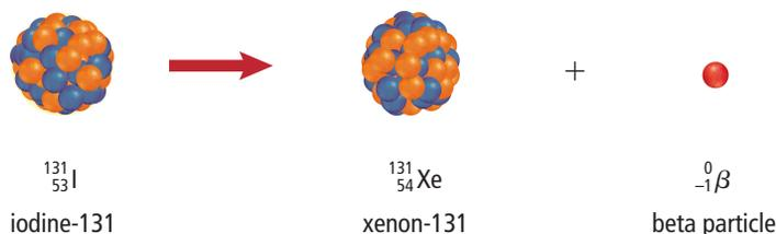
Figure 7.11 shows the decay of an iodine-131 nucleus, emitting a beta particle. The mass number stays the same, but the atomic number increases by one, producing the element xenon. The iodine-131 isotope is used in the treatment of cancer of the thyroid gland, a small gland in your neck that helps control how your body uses energy (Figure 7.12).
