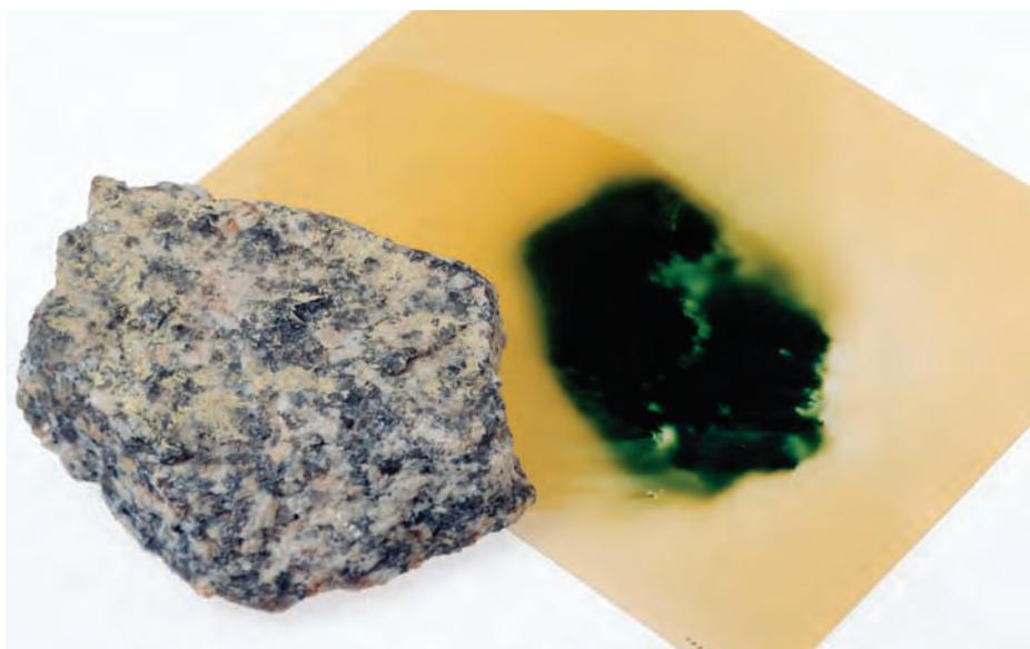
**Figure 7.2** A rock containing uranium salts causes photographic film to be exposed. This is evidence that the rock is radioactive. In this example, the radioactivity is coming from the uranium atoms in the rock.
