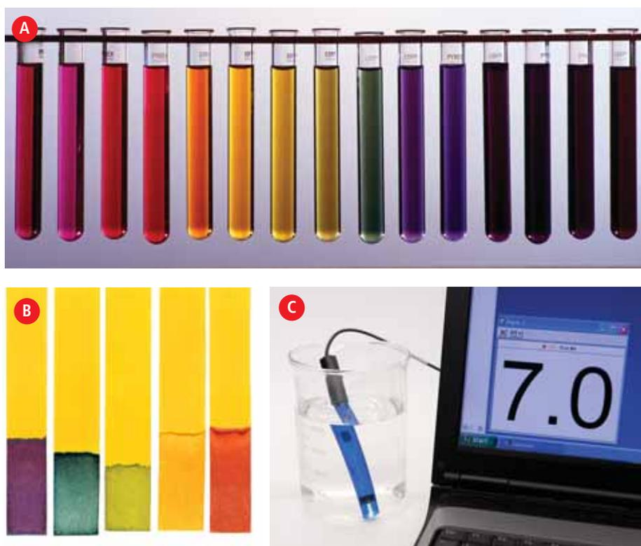
**Figure 5.4** Universal indicator can be prepared as a liquid and then dropped into a test sample (A), or it can be dried onto paper called pH paper (B). The sensor is measuring the pH of a solution (C).
