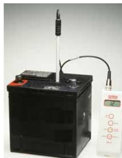
**Figure 5.7** The sulfuric acid in this battery has a pH of 1.2, which means it is extremely corrosive.
