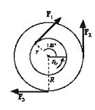
31. We assume clockwise motion, so the frictional torque is counterclockwise.
