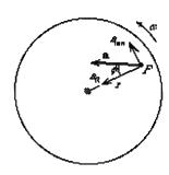
29. The force being applied by the rider is equal to his force of gravity. The maximum torque will be exerted when this force is perpendicular to the line from the axis to the pedal:
