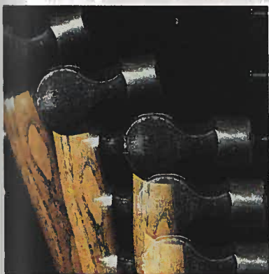
FIGURE 4-8 Multiflash photo of a hammer striking a nail. In accordance with Newton's third law, the hammer exerts a force on the nail, and the nail exerts a force back on the hammer. The latter force decelerates the hammer and brings it to rest.
