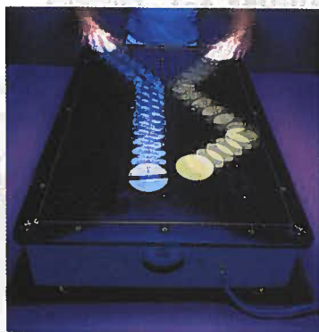
FIGURE 4-3 Photo of an air table. Air issuing from many tiny holes forms a thin air layer between the table and a puck, which, when given an initial shove, will travel at constant speed in a straight line (until it hits a wall or another puck).
