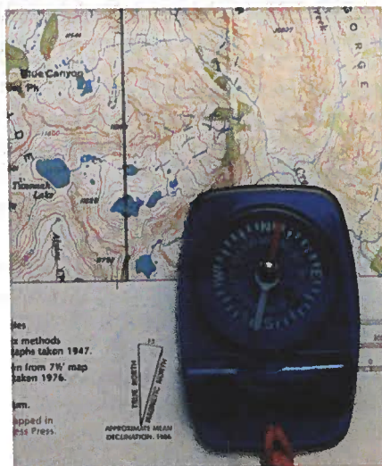
FIGURE 20-7 Using a map and compass in the wilderness. First you align the compass so the needle points away from true north (N) exactly the number of degrees of declination as stated on the (topographic) map: 15^\circ in the case shown. Then align the map with true north, as shown, not with the compass needle.
