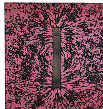
FIGURE 20-4 Thin iron filings indicate the magnetic field lines around a bar magnet.
